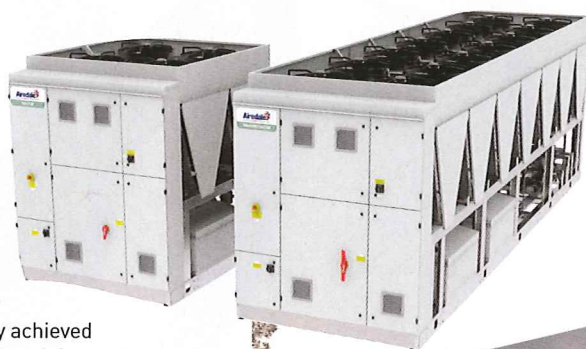
Exploiting the benefits of free cooling. Chillers such as Airedale's TurboChill (left) can utilise free cooling to generate energy savings of up to 50% compared with a conventional chiller. Indirect adiabatic air-handling units (below) provide a highly efficient external solution for data centres, freeing internal space as internal PAC units are not needed.
